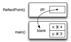
The parameter ptr is a reference to the structure named blank. The usual representation for a reference is a dot with an arrow that points to whatever the reference refers to.
